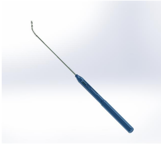
Figure 2.11: CAD model of second iteration prototype consisting of a pen-like handle.
