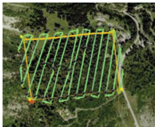
Figure 6.3 Sample UAS flight path for photogrammetry model (SPH Engineering, n.d.).
