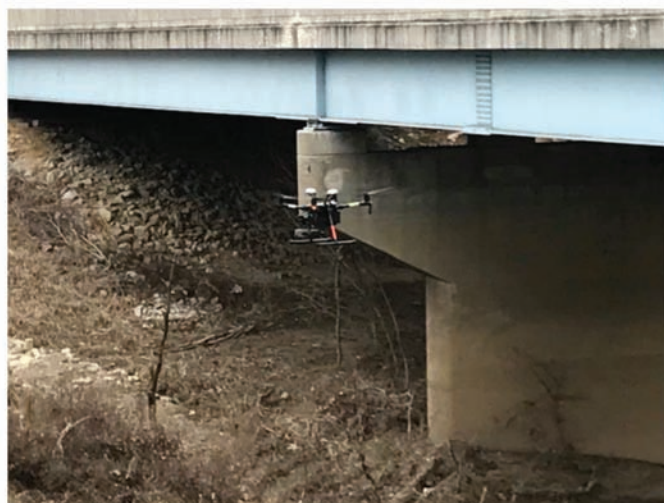
(b) UAS can document areas of bridge that are difficult to access (Fitzgerald, 2020).
