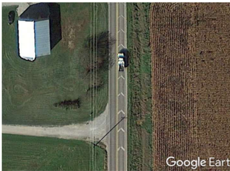
Chevrons prompting a speed limit (Corkle et al., 2001; Hallmark et al., 2007).
