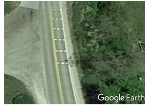
Transverse speed bars (Hallmark et al., 2013).
