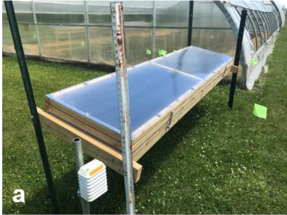
Figure 13. A passive solar dryer was constructed and tested on intact peppers at SROC in Waseca (a, b) and at a farmer-collaborator site (c). A smoker (d) was also constructed and tested for pepper drying at SROC. The SROC passive system was tested both outside and inside a high tunnel.
