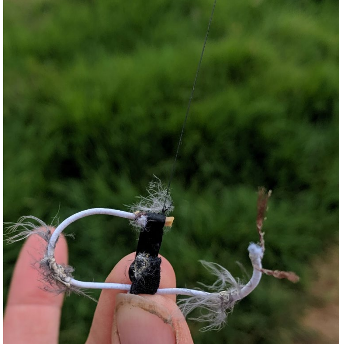
Figure 19. The recovered transmitter of WILD7 showing that he had untied the string in the weak link (rubber band), which eventually led to him to dropping the transmitter.
