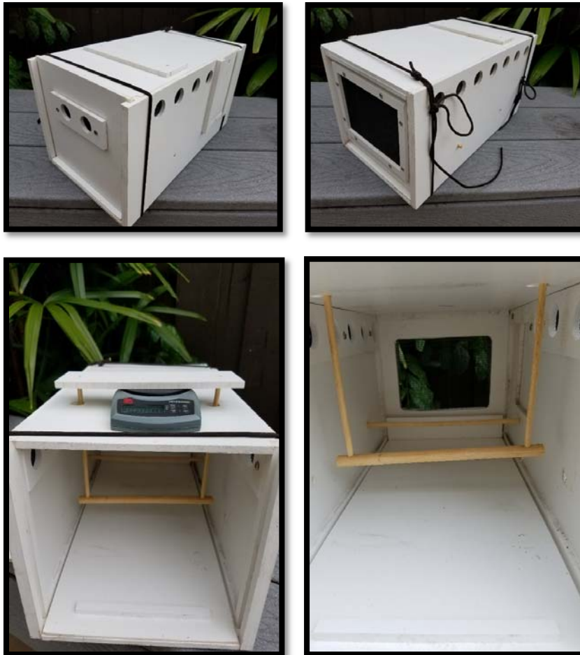
Figure 12. Kiwikiu (Maui Parrotbill; Pseudonestor xanthophrys ) single compartment holding cages to be used at the capture site's central camp with remote weighing system and removable perches and floor.
