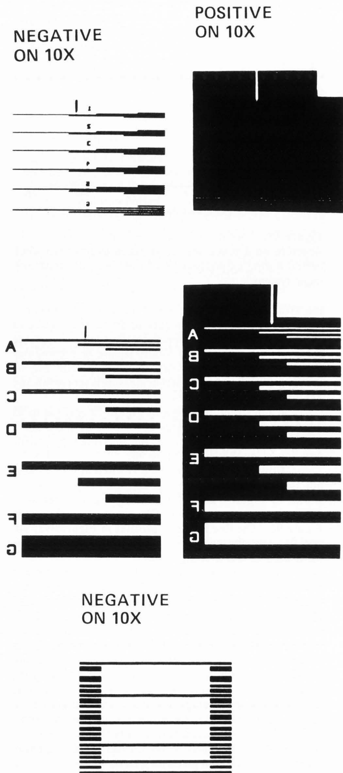
Figure 14. Basic patterns of the chrome-on-glass artifact consists of colinear single and multiple lines and spaces ranging from about 0.5 to 2.0 \mu\text{m} . (Reproduction of Figure 1 from Reference (48) courtesy of Dr. Hans R. Rottmann, IBM Corporation, East Fishkill, NY).
