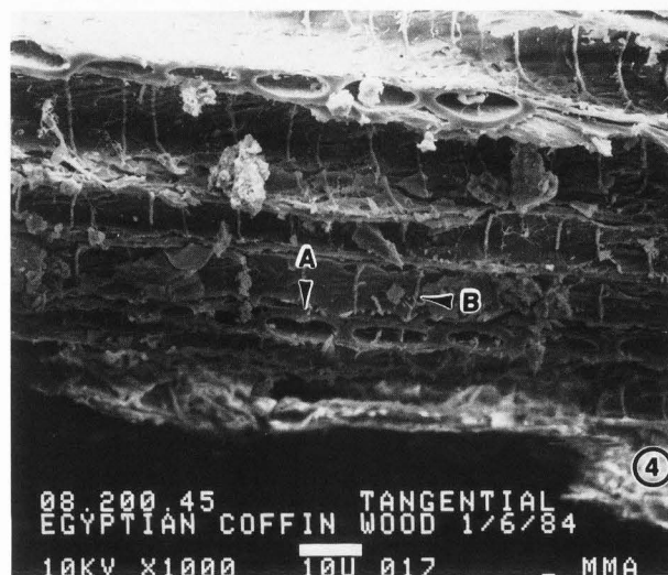
Figure 4. SEM micrograph of untreated wood sample (interior, cleaved surface) in tangential section, showing details of wood anatomy including uniseriate rays (arrow A), and helical thickenings (arrow B). Bar = 10 \mu m.
