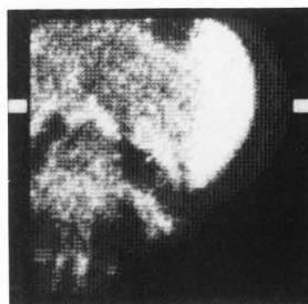
Fig. 12(a). Frontal PIXE image of the head in Ca X-rays stimulated by 4-MeV incident protons.
