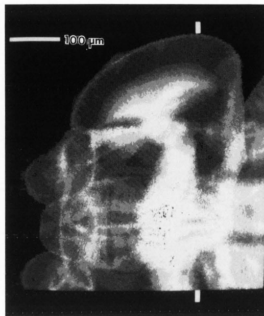
Fig. 2. A dorsal view of the head at twice the magnification of Fig. 1. The compound eye is at the top of this figure; the antennae are visible at the left. The dense central brain is transparent almost everywhere to 4 MeV protons in this view. The short vertical bars above and below locate the five scans of Fig. 5.
