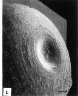
Figs. 4a & 4b. Using a copper rod and a slurry of emery produces a characteristic leading edge when drilling hard stones such as agate. In these impressions, the central depression would be an elevation in the substrate. It is relatively smooth and represents the site of preferred wear in the drill itself. Bar =  $500 \mu m$  and  $250 \mu m$  respectively.
