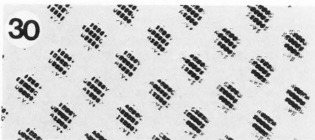
Figure 30. Computer generated lattice image of the calcite [421] zone at defocus = -65 nm. (Parker et al. 1983).
