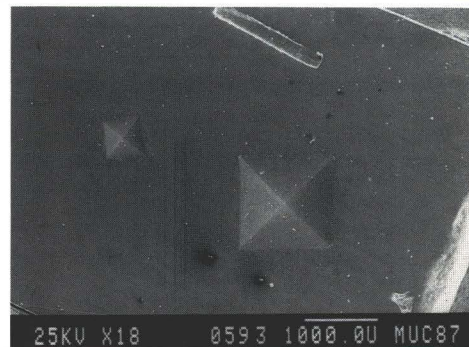
Figure 10. Two hardness indentations of different depths are made on a parallel-sided zinc specimen
