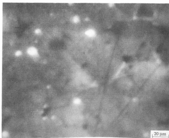
Figure 9. CL micrograph from sample R2 annealed in a strongly reducing atmosphere at 293K.
