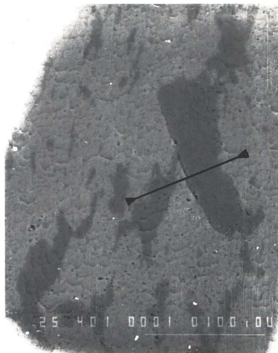
Figure 3. Backscattered electron image of microcline perthite. Horizontal field width is 300 \mu\text{m} . Albite exsolution (dark) lamellae in a K-feldspar matrix (light) are visible. Dimensions of large lamella parallel and perpendicular to black line are approximately 30 \times 140 \mu\text{m} .
