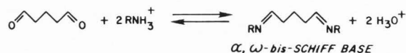
Figure 1. Bis-Schiff base formation. Schiff base formation is rapid and reversible in aqueous solution. Acid is a byproduct near pH 7 (19).
