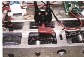
Figure 2.7: Vehicle with the kill switch in the off (horizontal) position.
