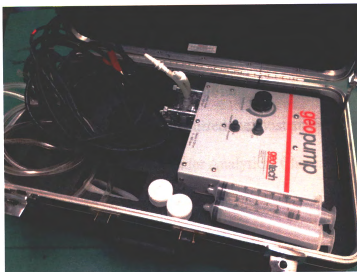
Figure 3. Peristaltic pump and syringes used to contrast filtering methods.
