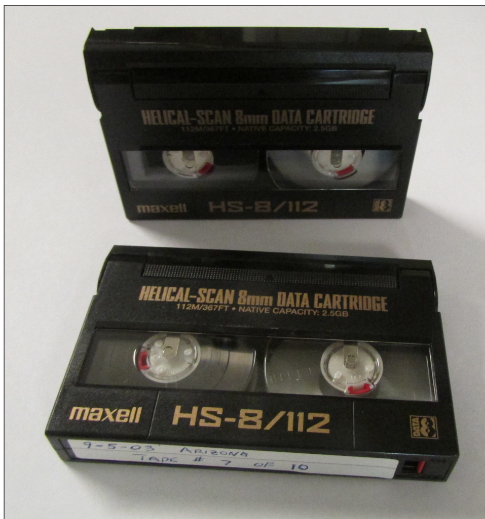
Figure 4: Photo of 8 mm magnetic tape cartridges, similar to the ones used to store the original 2000 lidar point clouds.
