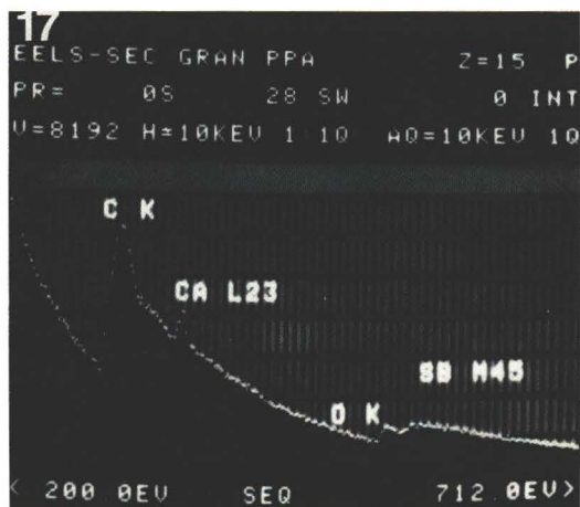
Fig. 17. Electron energy loss spectrum of CaPA deposits in the secretory ameloblast, showing separate edges from calcium (Ca L23) and antimony (Sb M45).
