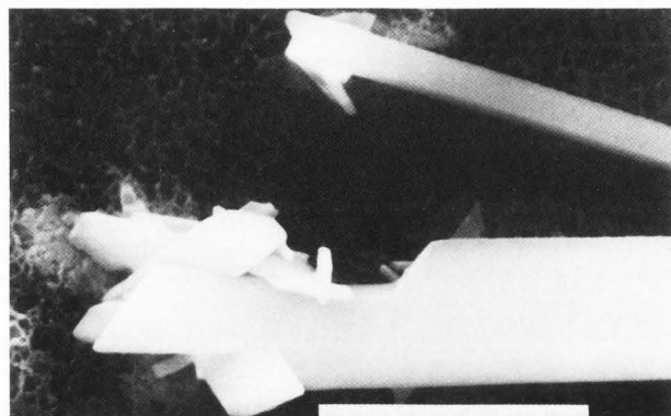
Fig.11. Scanning electron micrograph of calcium sulfate induced by barium sulfate seed. Note the typical twinned crystals formed between calcium and barium sulfate observed in all experiments (Table 3). Bar = 10 \mu m
