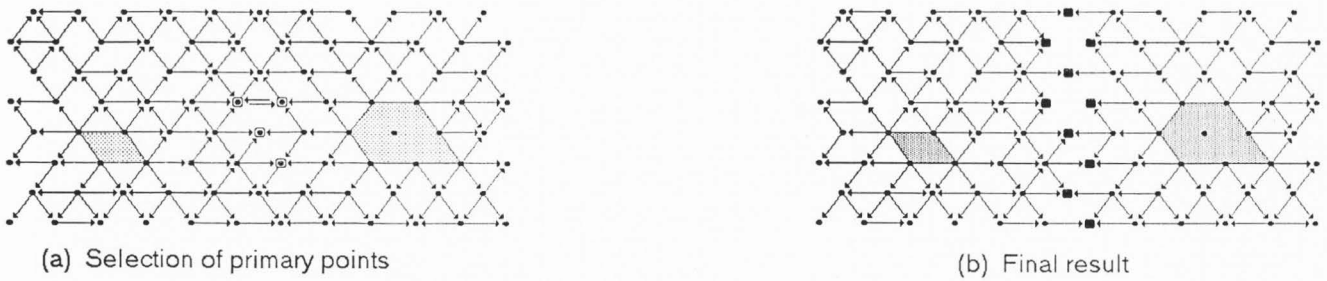
Figure 9. Watershed by arrowing: primary divide points (a), final result (b).
