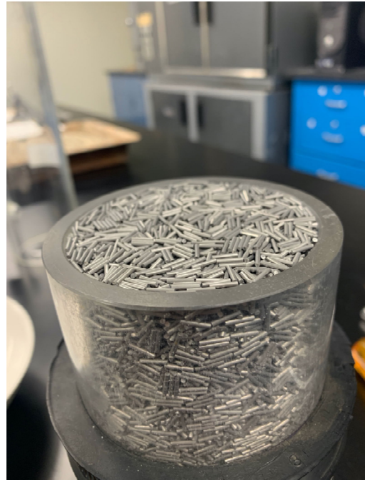
Figure A7. Stereograph photos of Stainless Steel Pins and sample shown in permeameter tube
