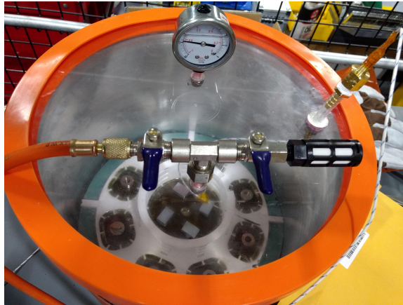
Fig. 6.10: Picture of vacuum potting setup.
