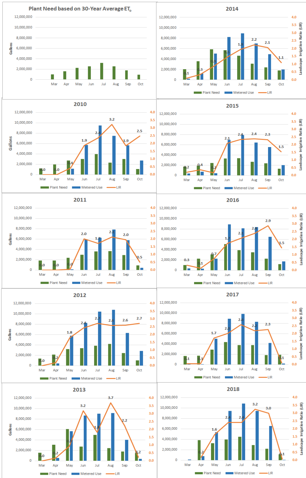
Figure 9. WaterMAPS™ monthly analysis for Utah State Capitol by year (2010 – 2018) with reference to 30-year average (1979-2008) ET o -based plant water need. Each annual panel shows plant water need (green bars) compared to metered water use (blue bars) with LIRs (orange lines and numbers).
