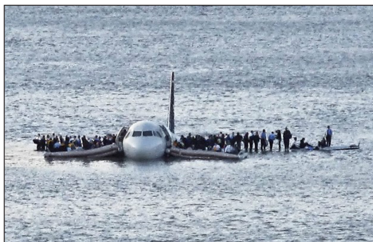
Figure 1. On January 15, 2009, U.S. Airways Flight 1549 (Airbus 320), with 155 persons aboard, made a forced landing in the Hudson River after ingesting Canada geese ( Branta canadensis ; mean mass >3.8 kg) into both engines. The strike occurred at about 870 m above ground level and 8 km from LaGuardia Airport, New York, USA, where the aircraft had just departed. This incident highlights the risk to aviation posed by large, flocking species of birds, especially at altitude outside the airport boundaries where traditional wildlife management techniques are not effective. Most turbofan engines are not certified to withstand the impact of birds with a mass >1.8 kg and none are certified for birds >3.6 kg (photo courtesy of S. Day, Associated Press).
