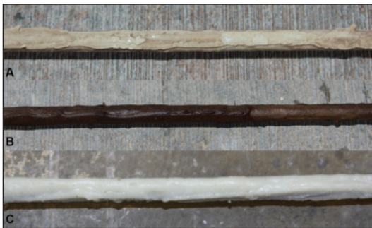
Figure 5. Anthraquinone-treated and no-anthraquinone-treated aluminum perches used for repellent efficacy testing with European starlings ( Sturnus vulgaris ) at the National Wildlife Research Center's Outdoor Animal Research Facility, Fort Collins, Colorado, USA, 2016–2018. (A) Airepel® HC with castor oil formulation; (B) Airepel HC with castor oil without anthraquinone formulation; (C) MS2 formulation (photos courtesy of H. McLean).
