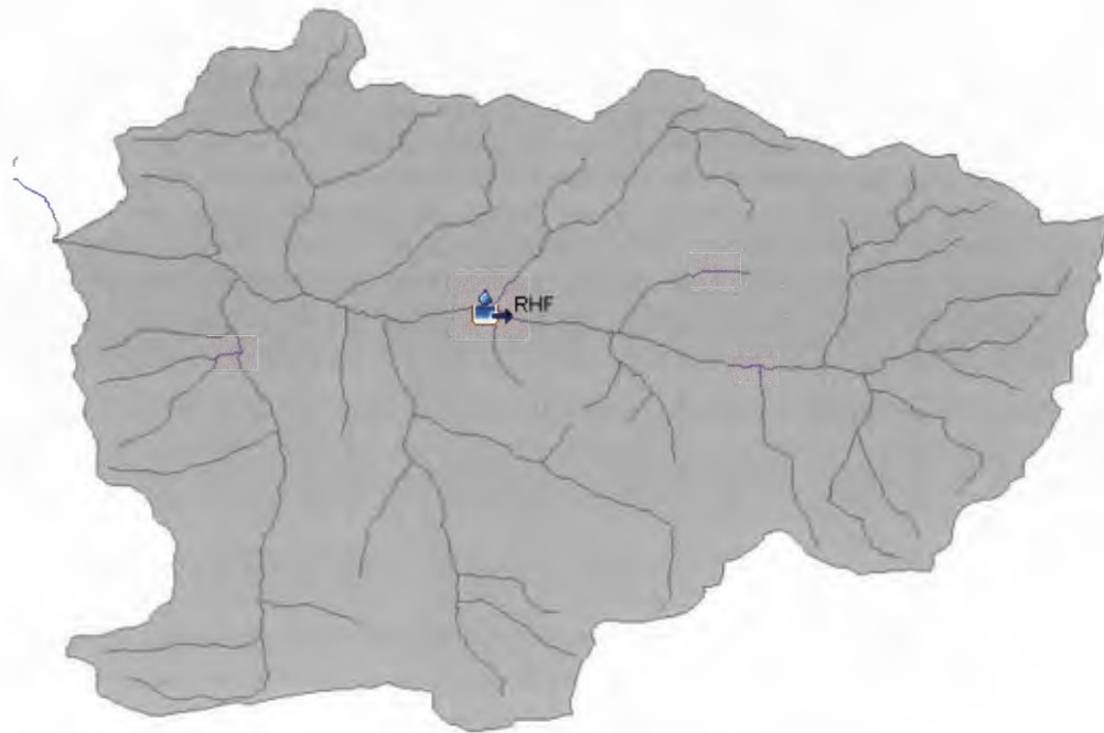
Figure 9. Basin model for HEC-HMS model.
