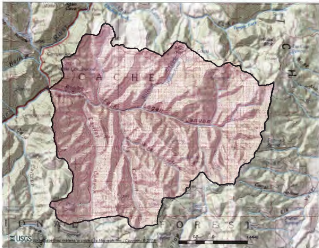
Figure 8. Watershed delineation from USGS Streamstats.
