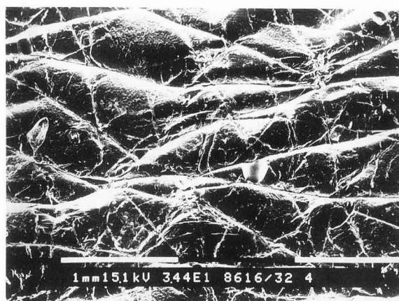
Fig 2. Positive replica of a lower arm skin surface (gold-sputtered Araldite (R)) obtained from a (dental) silicone plastic negative imprint of the skin.
