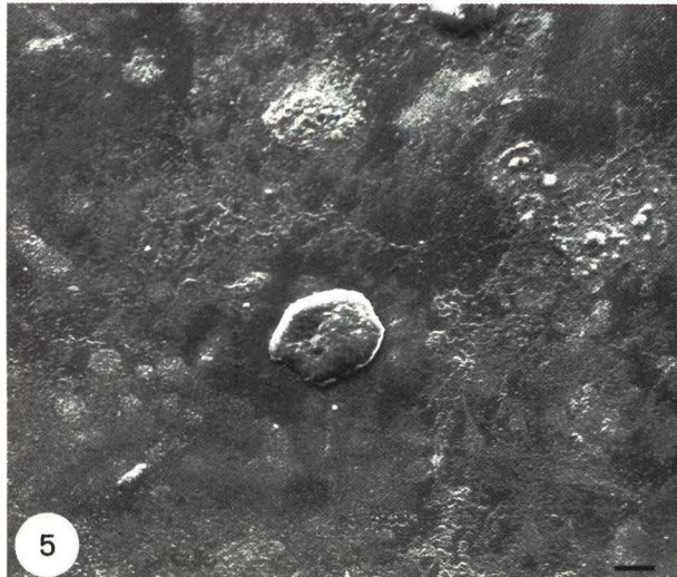
Fig. 7. Continuously worn SCL, fixed specimen. A deposit with an unusual ferning-like appearance is evidenced. SEM. Bar = 100 \mu m
