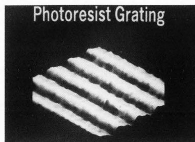
Fig. 9: Image of a photoresist grating by AFM; line-width = line spacing = 100 nm, photoresist thickness = 90 nm.
