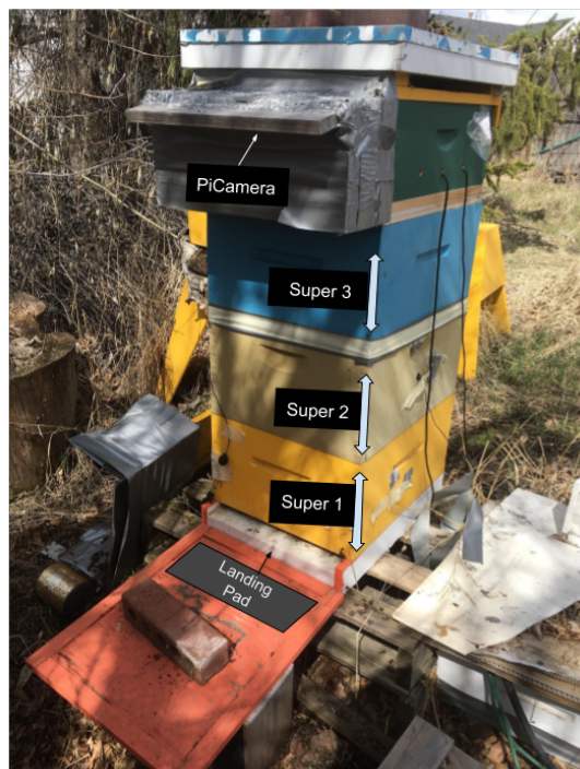
(a) A BeePi monitor box on top of a Langstroth beehive that consists of 3 supers; the camera is protected against the elements with a specially constructed wooden box.
