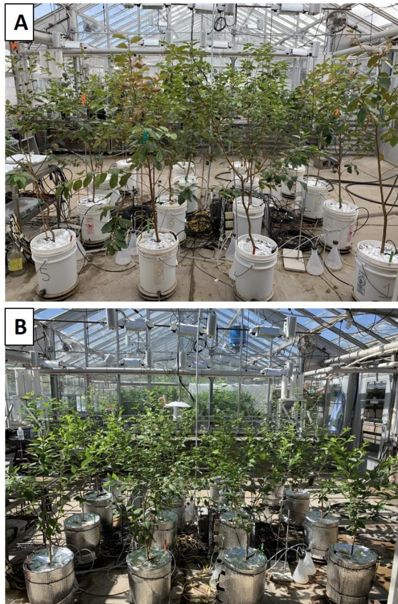
Fig. 4.2.1. A 16-cell lysimeter system used to assess transpiration rates for Krymsk ® 5 and 6 rootstocks for the first (A) and second (B) drought trials.
