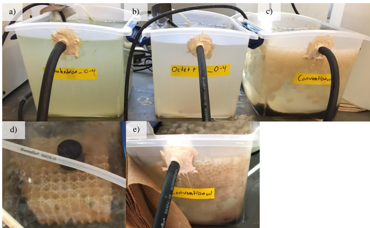
Figure 5-10: Images depicting settled biomass in the conventional carriers reactor. Images a-c depict the Octahedron-0.4 mm, Octet + Simple Cube-0.4 mm, and the Conventional. Carriers, respectively after startup (1000 mg/L COD). Images d-e depict the Octahedron-0.4 mm and the Conventional Carriers, respectively after visible biofilm has developed on the carriers (100 mg/L COD). Note that in both cases, the Conventional Carriers had large quantities of black, settled biomass.
