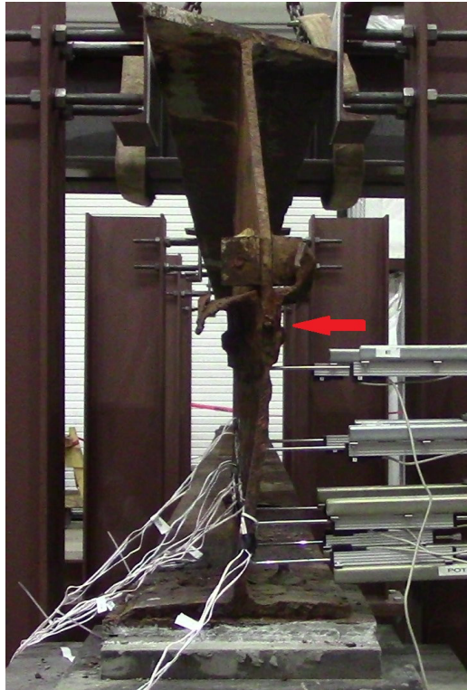
The image above shows an example of a web deviating from straightness
