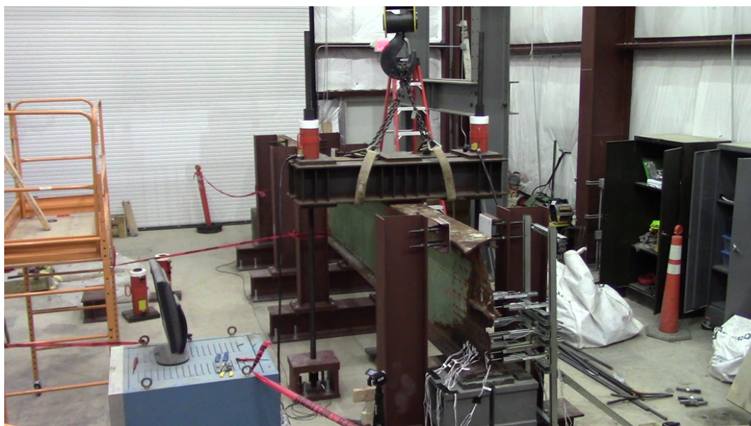
The Brack Lab at UMass Amherst: Setup for Tests Conducted on Corroded Steel Bridge Beams Taken from Decommissioned Bridges in Massachusetts.
