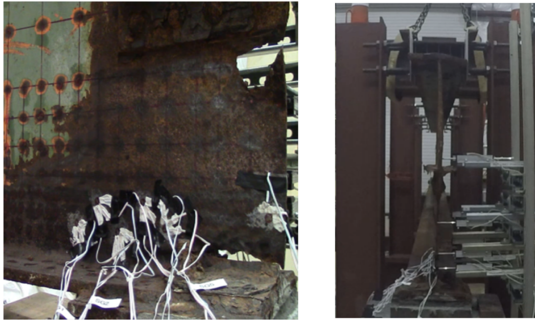
Figure 4.2: (Left) Strain Rosettes (Right) Linear Potentiometers
