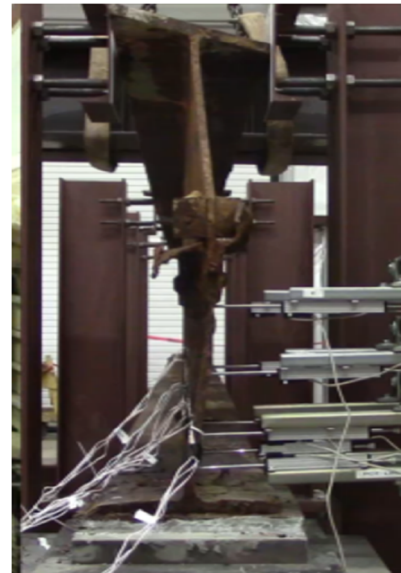
Figure 4.11: (Left) Strain Rosettes (Right) Linear Potentiometers
