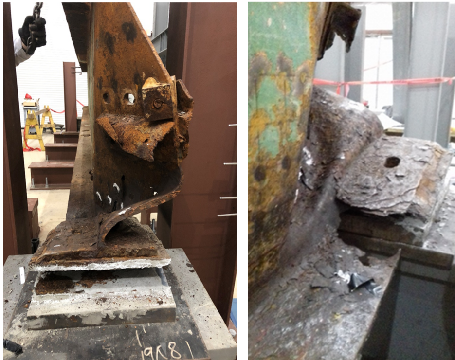
Figure 4.18: Residual Deformation of Corroded Web End
