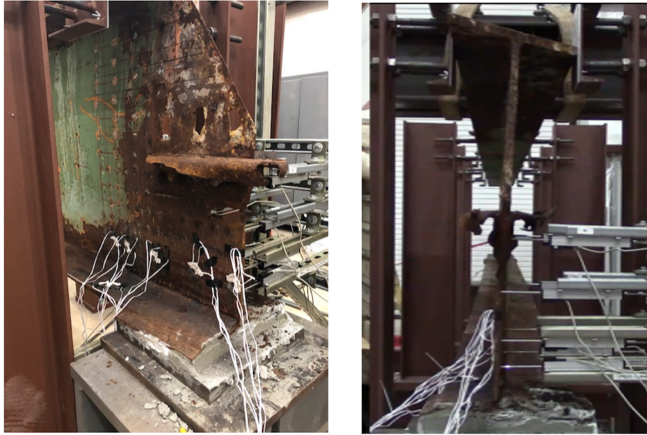
Figure 4.20: (Left) Strain Rosettes (Right) Linear Potentiometers
