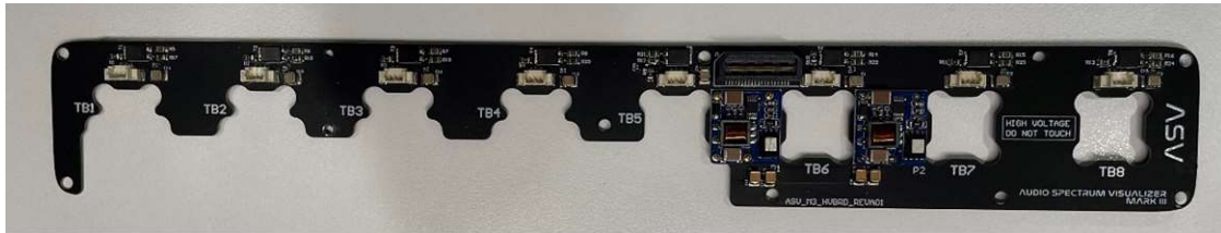
Figure 20 --- High Voltage Board PCB & DC/DC Flyback Power Modules
