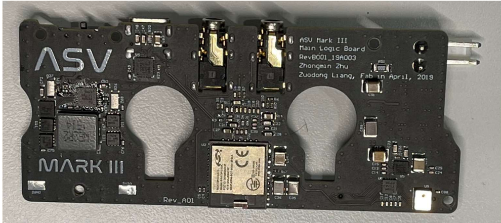
Figure 17 --- Low Voltage Controller Board
