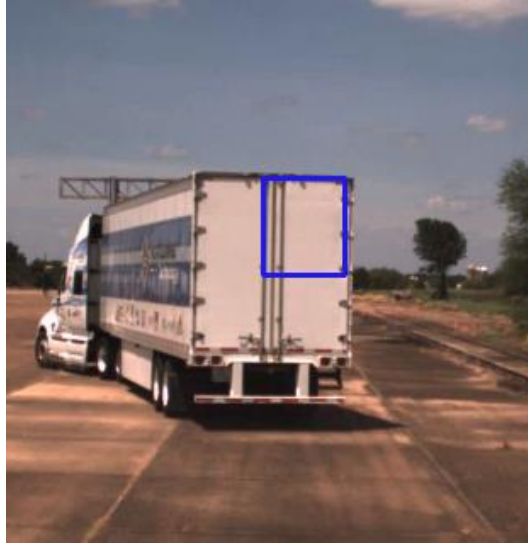
Figure 31: False detection during simulated testing for control algorithm
