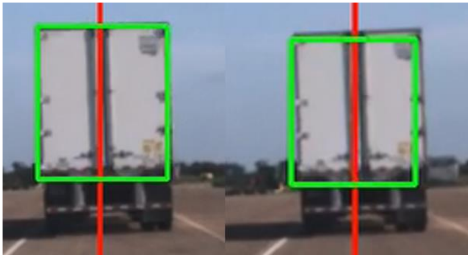
Figure 45: Normal variation in detected size between frames
