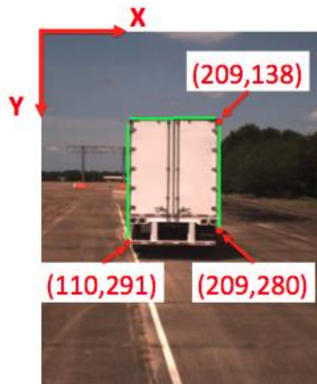
Figure 6: Axis definition with example (x , y) pixel coordinates
