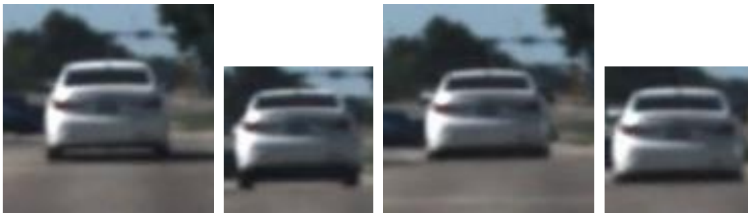
Figure 20: Size variability in Haar cascade detection between successive frames
