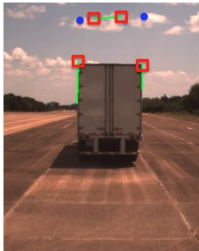
Figure 11: Failed detection: The calculated intersection points do not lie within the feasible region
