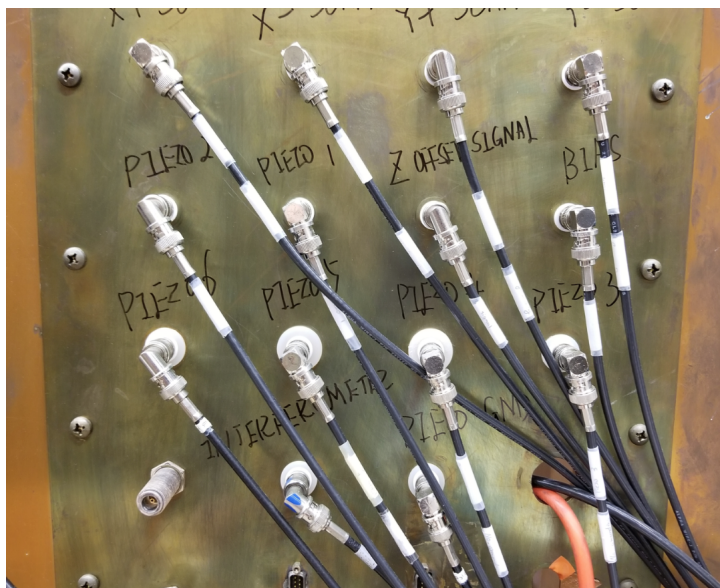
Figure 2.19: BNC cables carrying STM control voltages.
