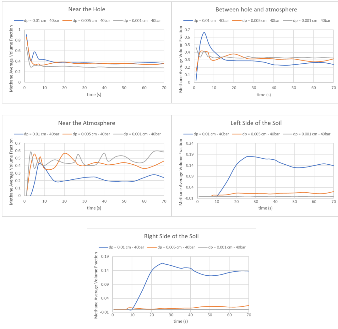
Figure 33: Methane average volume fraction with time for the different particle diameters at 40 bars
