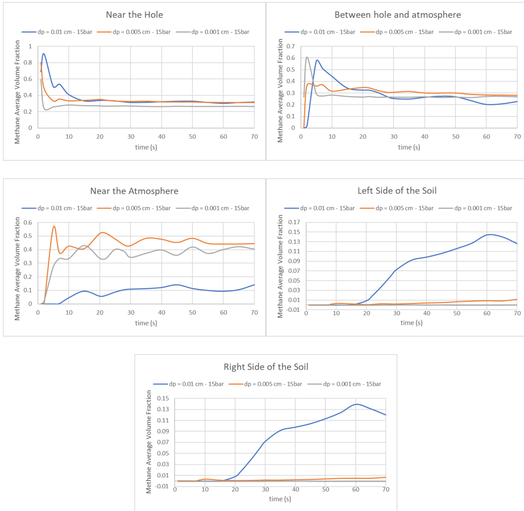
Figure 31: Methane average volume fraction with time for the different particle diameters at 15 bars
