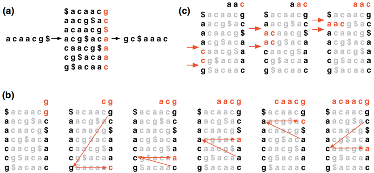
Figure 2.5: (a) Burrows Wheeler Transform, (b) Recovering T from BWT(T), (c) Backward search for pattern aac [4]
