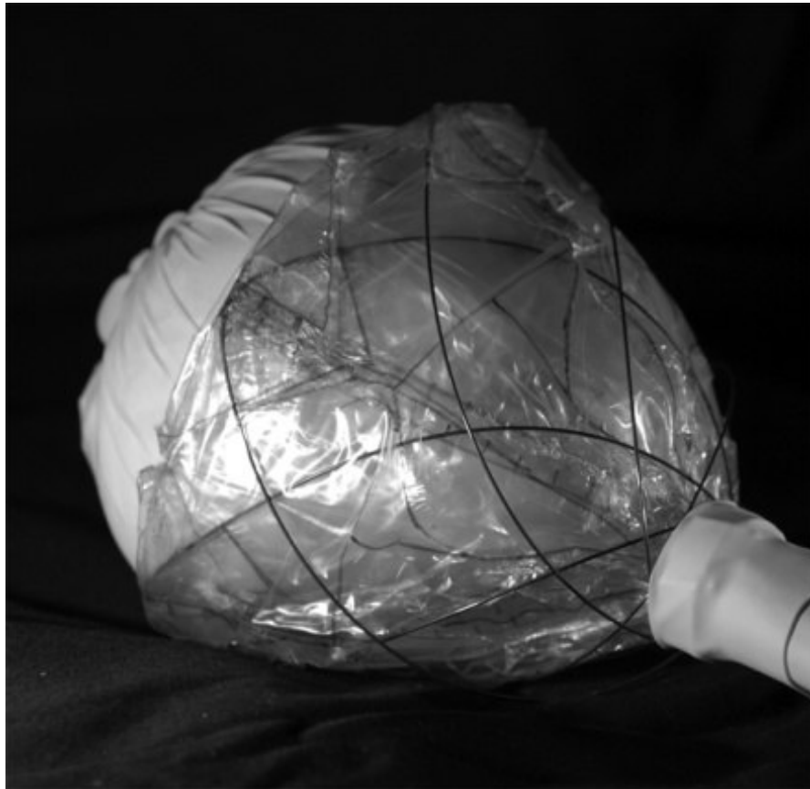
FIGURE 14: Minimally Invasive Simultaneous Function Device. A prototype of the minimally invasive device capable of simultaneous passive support and active assist, deployed about an excised ovine heart that is preserved and wrapped in thin latex for handling.
