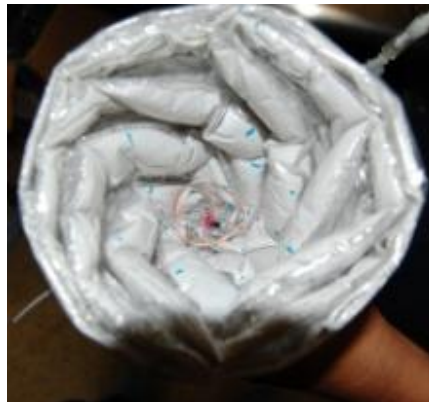
Fig. 6. Helical passive bladders forming the cup interior of a previous prototype.
