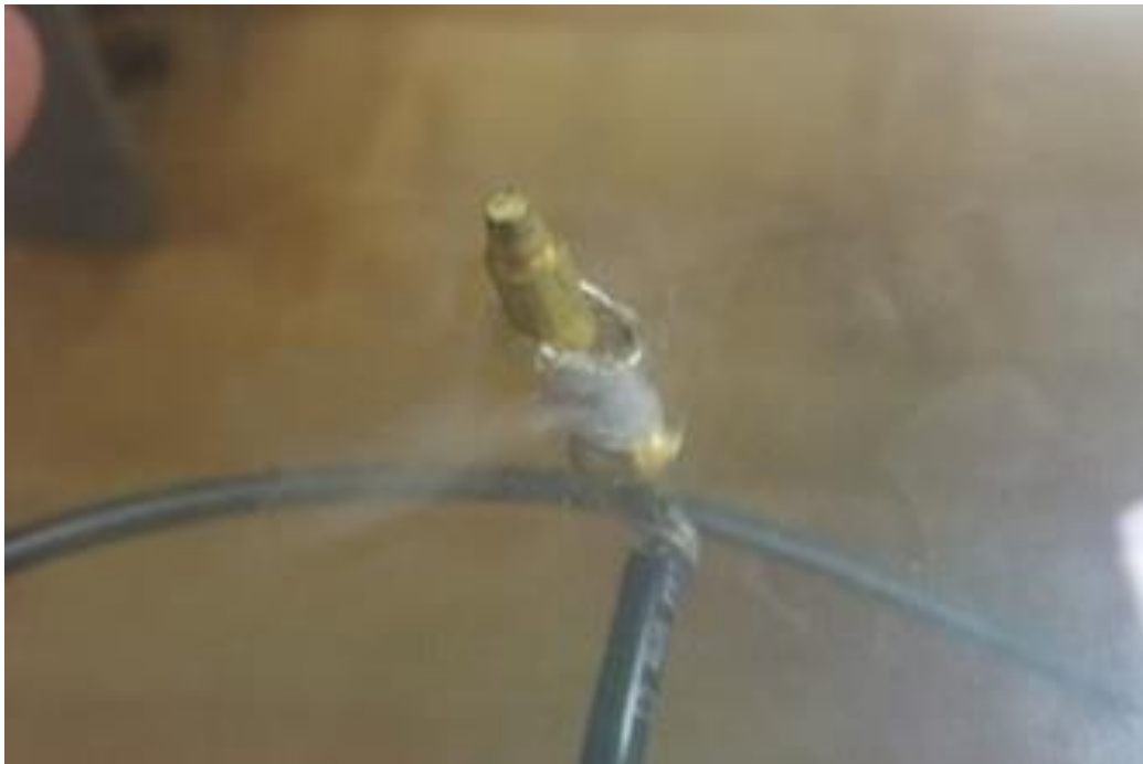
Figure 30: Melted mounting plate on the first generation AG.
