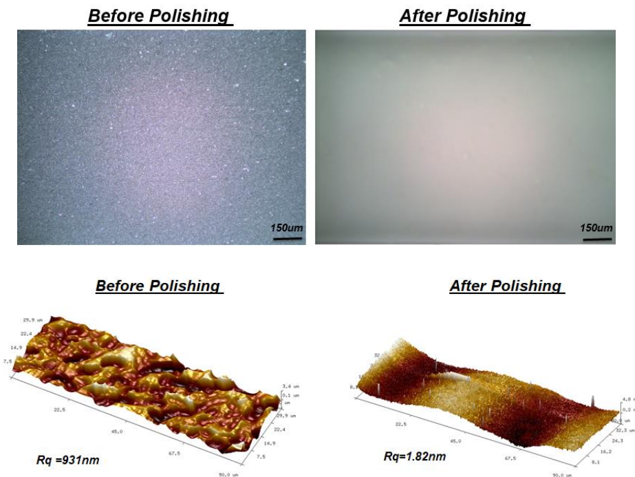
Figure 59. Microscope and AFM images of rough surface before and after polishing
