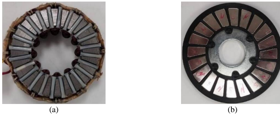
Figure 23. (a) Tape Wound Stator and (b) Rotor of Axial Flux PM Machine
