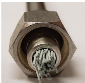
Figure 1-4. An example lab scale fiber sorbent module, packed parallel to the flow direction
