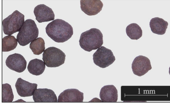
Figure 2.7 Optical microscopy image of Carbolead CP 30/60 particles from an optical microscope (Leica, USA).
