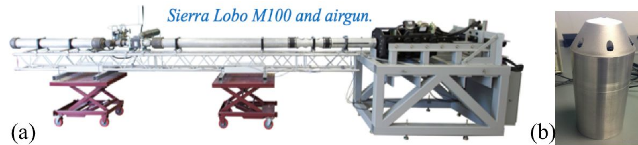
Figure 4: Facility at Sierra Lobo for impact tests. (a) M100 and airgun assembly used to accelerate and impact the impactor capsule. (b) Test article body/impactor capsule.
