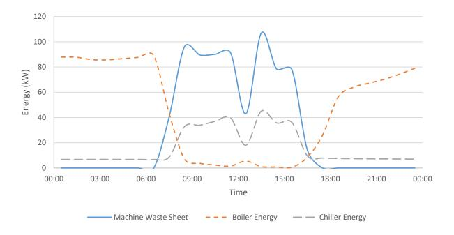
Figure 4- Waste heat output from machinery alongside energy required for boiler and chiller systems
