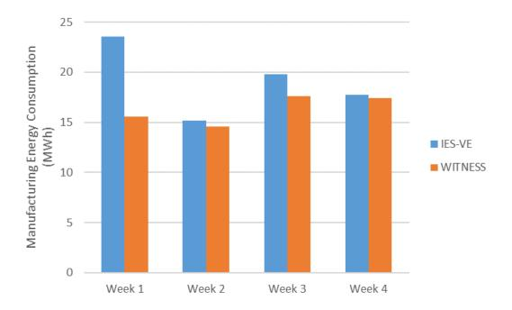
Figure 3-Weekly Manufacturing Energy Consumption from IES and WITNESS
