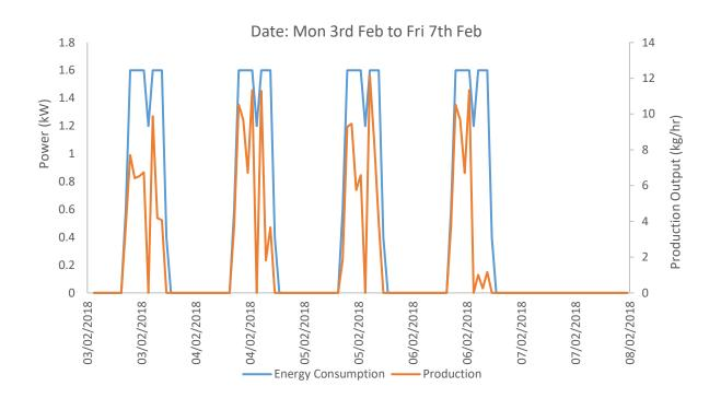
Figure 7 - Energy Use VS Production Output for Bumotec Turrnmill
