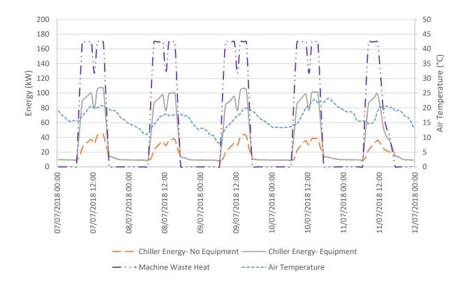
Figure 6- Chiller energy requirements for a the facility with and without equipment, plotted alongside outdoor air temperature and machine waste heat
