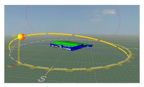
Figure 2- Building model in IES-VE, displaying the solar path around the building
