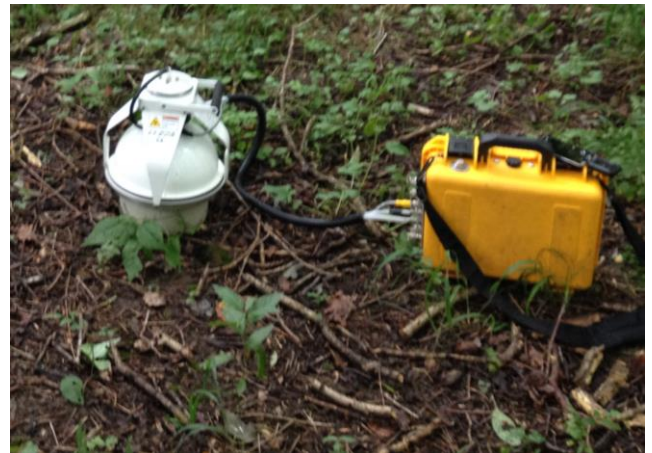
Figure 2.3. Photographs of mesocosms in the field and field CO 2 efflux measurements. a) Mesocosm in an oak stand, showing the wire-mesh hat to prevent natural litter inputs. b) The LiCor L1-8100A survey system during a soil CO 2 efflux measurement.
