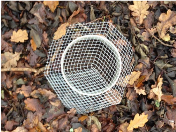
Figure 2.3. Photographs of mesocosms in the field and field CO 2 efflux measurements. a) Mesocosm in an oak stand, showing the wire-mesh hat to prevent natural litter inputs. b) The LiCor L1-8100A survey system during a soil CO 2 efflux measurement.
