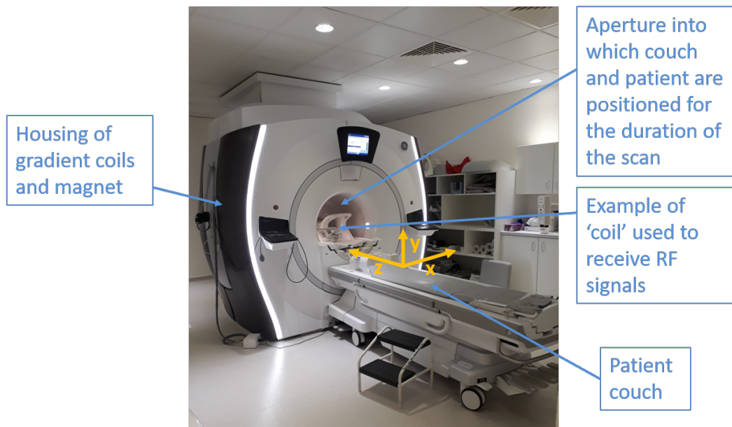
Figure 2.12: An example MR scanner showing the various typical axes and directions, and the location of the different parts of the scanner.
